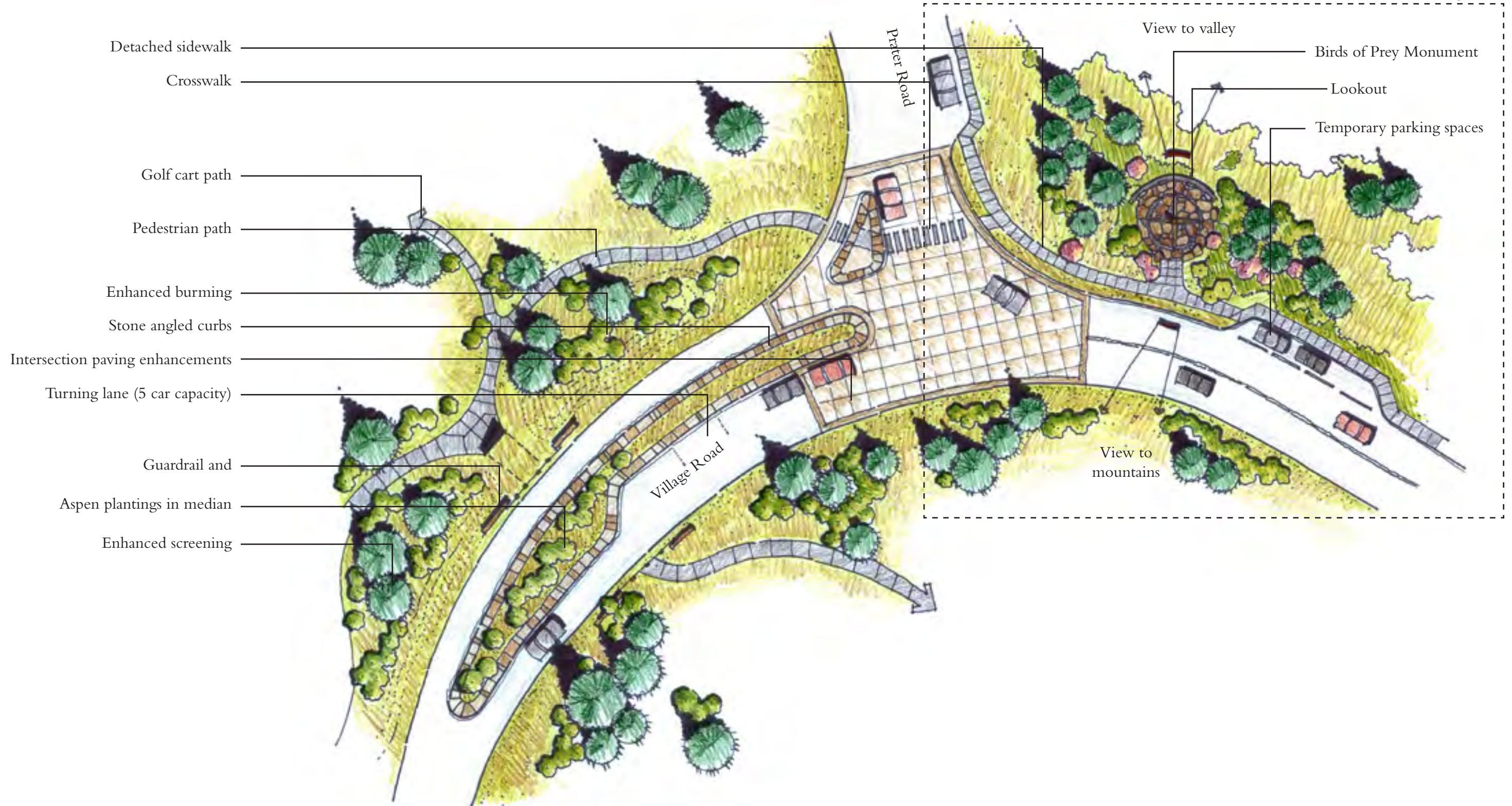
PROPOSED PLAN VIEW SHOWING ENHANCEMENTS AT THE VILLAGE ROAD AND PRATER ROAD INTERSECTIONS
